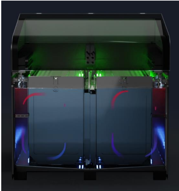
Figure 13: heat circulation within the immersion tank.
