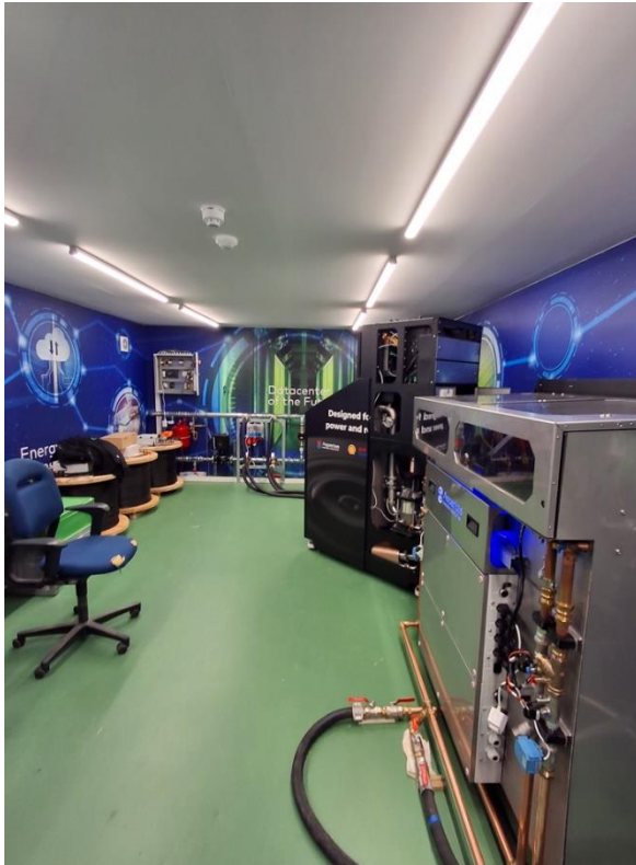
Figure 1: The staging lab environment, equipped with immersion tanks, control equipment, and the cooling cycle components.
