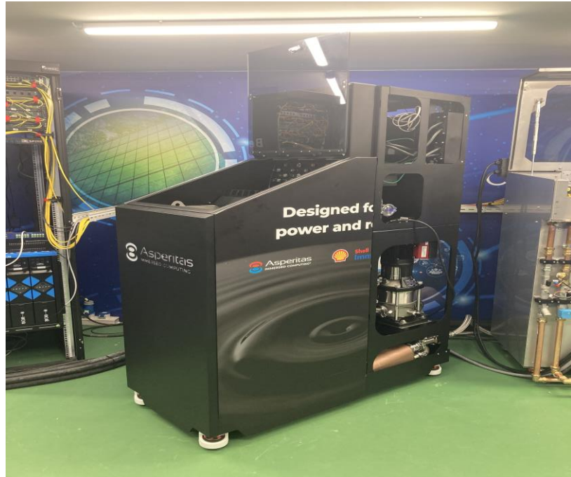
Figure 16: : Asperitas DFCX1 immersion tank.
